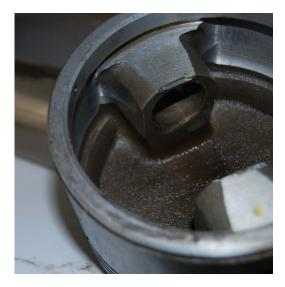
In addition to the inferior molding, whoever prepared the pistons in my plane attempted to establish and equalize required weight by grinding out material inside some pistons with a hand-held die grinder and bounced it all over the insides of the pistons. The photo below is typical. No wonder cracks started with all those stress risers being pounded.
