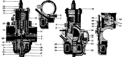
fuel needle spring is not compressed by the float weight. It is therefore advisable to put the carburettor in a horizontal position until the float just contacts the float needle. In this position the pointer on the float hinge is set in such a way that the float top edges are parallel to the top edge of the float chamber.
