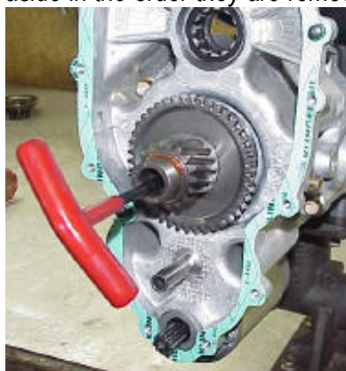
Figure #3 – A long reach Allen wrench is need to remove the bolt hidden down inside the small drive gear.
