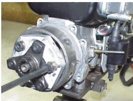
Figure #5 – In order to change the crankshaft, the spider, hardy disk, and flywheel need to be removed. Note fixation bolt in pulse port to prevent crank from turning.
