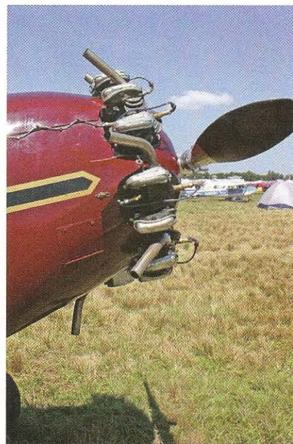
This RNF began life with a 110-hp Warner, but today it has a 145-hp Warner
