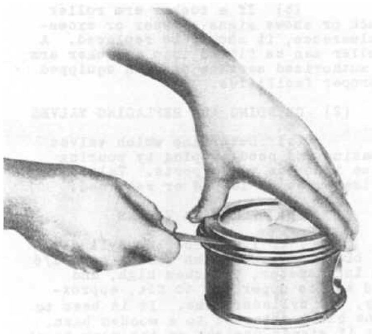
Figure 4. Checking Piston Ring Side Clearance in Piston.
