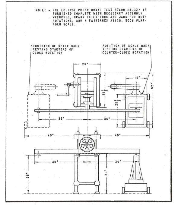
Figure 3—Prony Brake Test Stand for Testing Starters
