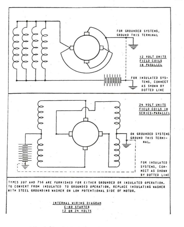
Figure 1- Schematic Internal Wiring Diagram
